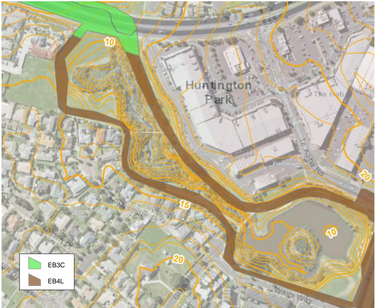
Figure 15. Topographic contours in and near EB4L, 5 m elevation intervals. Source: Project GIS.
